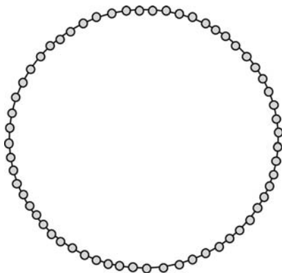
FIGURE 15.4. An example of a regular network. This network is a ring of nodes in which each node has a link to its two nearest neighbors.
